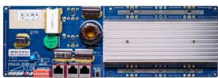
RS485 Communication between battery and inverters Band rate:9600ps RS485 Interface Communication between parallel packs or BMS and PC Band rate:9600ps
