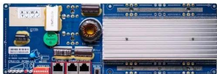
RS485 Communication between battery and inverters Band rate: 9600bps RS485 Interface Communication between parallel packs of BESS and PC Band rate: 9600bps
