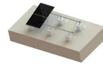
TRIANGLE FLAT ROOF SYSTEM
