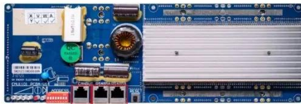
RS485 Communication between battery and inverters Baud rate:9600bps RS485 Interface Communication between parallel packs or BMS and PC Baud rate:9600bps
