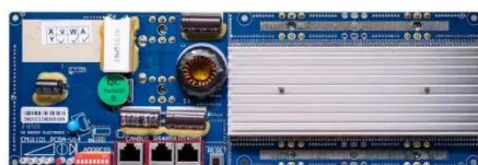
RS485 Communication between battery and inverters Band rate:9600ps RS485 Interface Communication between parallel packs or BMS and PC Band rate:9600ps
