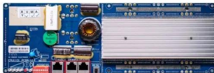
BS485 Communication between battery and inverter Band rate: 9600bps BS485 Interface Communication between parallel packs of BMS and PC Band rate: 9600bps
